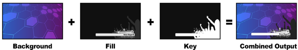
Combining a background, fill and key in a linear key
